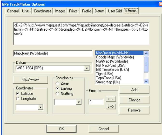
GPS TrackMaker® can be configured to open the Internet Explorer®, Netscape Navigator® or other similar program, allowing to show the position of a Waypoint, Tracklog or Route segment on a map.
