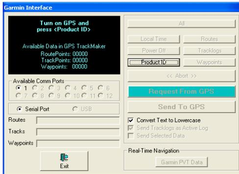
To activate real time navigation in Garmin® Models, open the **Garmin Interface** window through the *Interface* menu, and do the GPS recognition through *Product ID* button and then press *Real Time Navigation* button.
