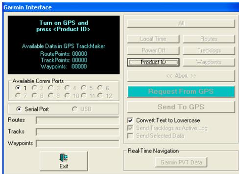
The communication between the PC and the GPS is very easy with the **GPS TrackMaker®**. Just open the specific window for your GPS model, clicking on the *Interface* menu. Then, turn on the GPS.
