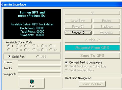
To set the PC's internal Clock, just click on the **<Local Time>** button located in the *Garmin Interface* window so the date and time stored in the GPS will be transferred to the PC clock. For that, it is necessary that the program recognizes the receiver; if not, this button will be disabled. To configure the local time, see [Configuring Local Time](#).
