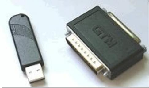
The Hardware Key or *dongle* is an electronic plug that works as an unlock password of the GTM PRO®. The plug is easily connected to the printer port or USB port, and must be present when GPS TrackMaker Professional® is being executed.
