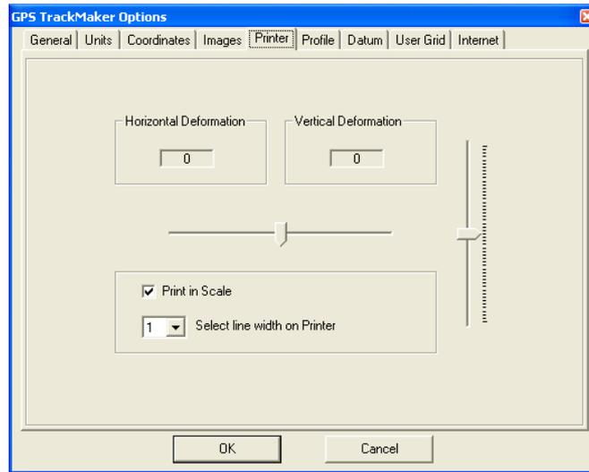
Every time a map is printed, the program automatically configures the printer to the scale indicated on the screen.
